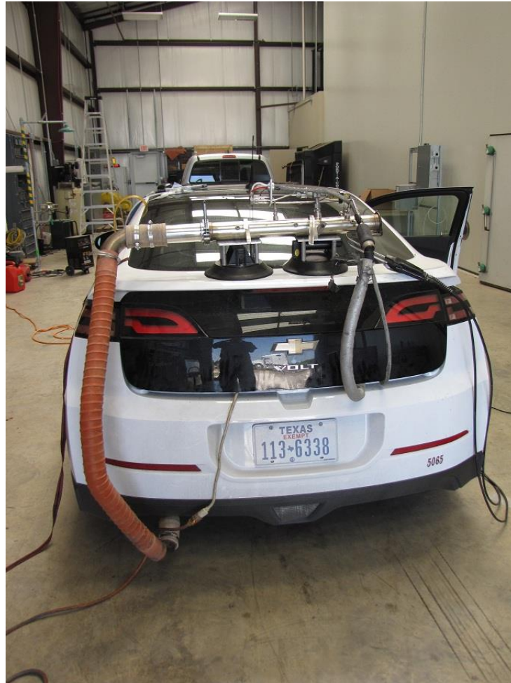
Figure 2: Test Vehicles in Chamber for Battery and Idling Testing.
