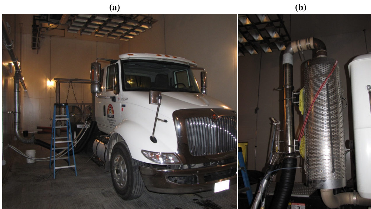
Figure 1. A Test Vehicle (a) and Sampling Lines Installed on Exhaust of a Test Vehicle (b).
