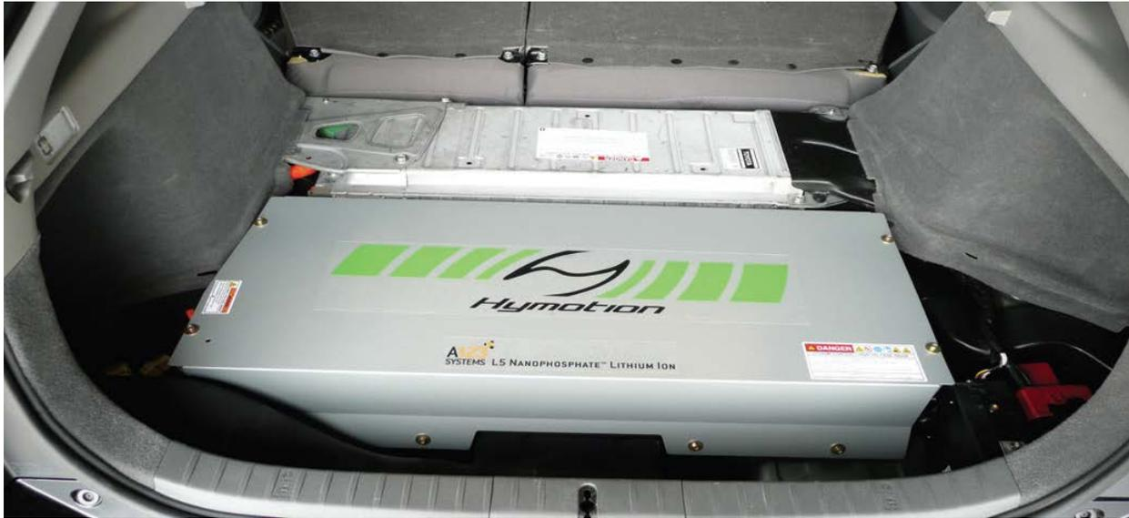
**Figure 1: Pictures of a Test Vehicle and a L5 PCM; (a) a test vehicle and (b) L5 PCM installed on the vehicle.**
